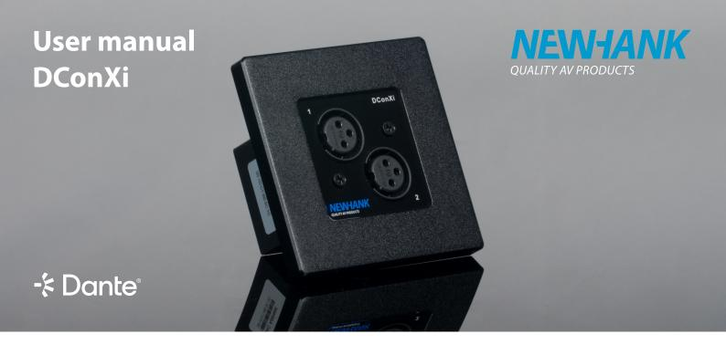
This two-channel XLR input panel converts analog audio to Dante. Each input is equipped with an adjustable preamp that offers up to 42dB of amplification plus -100 to +27dB digital gain, along with switchable Phantom Power for handling microphones and other audio sources with precision. DConXi also provides an API for integration with third-party control systems, making it an ideal choice for customized installations.
